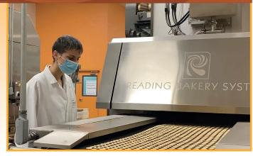
RBSConnect also monitors production in real-time and manages a Closed Loop Oven Control System that captures data on product flow rates, temperatures, energy efficiency trends, and other Key Process Indicators. Ultimately, the system helps ensure a higher percentage of in-spec product and less waste on the line.
