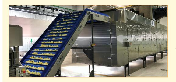
After baking, the chips are fed into a 3-Pass convection dryer that efficiently reduces the product to its final moisture.
